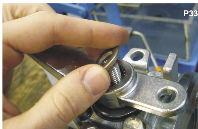
Replace the M12 washer.
