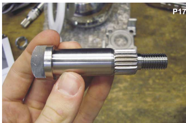
Examine the valve spindle for damage along the diameter where the seal will be located.
