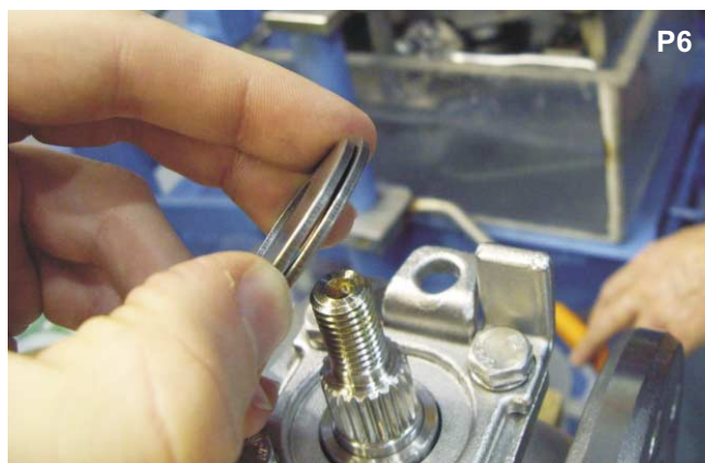
Remove the two Belleville washers noting the orientation.
