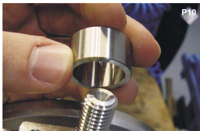
Remove the top stuffing bush.
