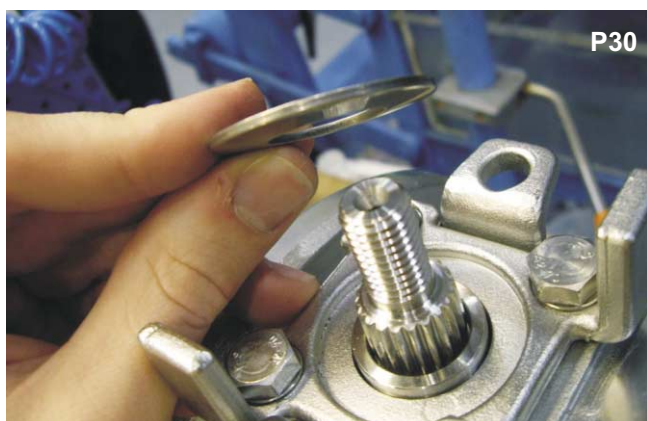
Replace the first Belleville washer, this must be placed dished side down as shown.
