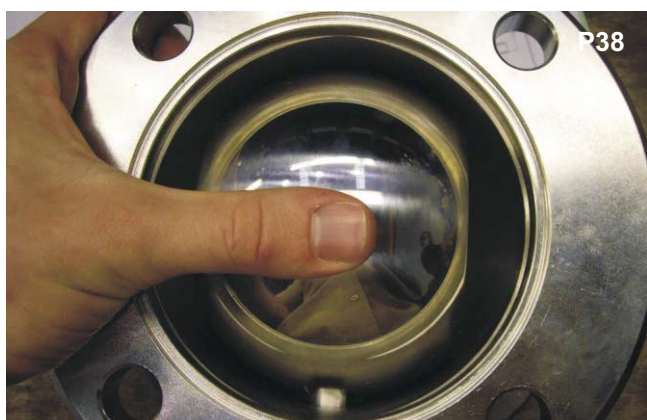
Slight adjustment of the stuffing clamp may be required to ensure the ball is correctly aligned in the valve body and seats. Once adjusted fully tighten up the clamp plate bolts which had previously been hand tightened using a 13mm A/F wrench.
