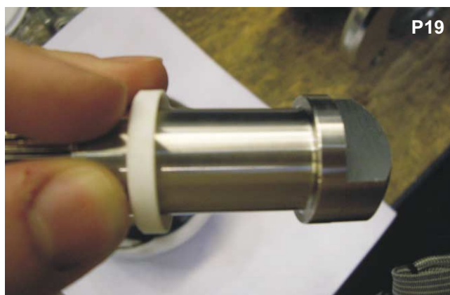
Slide the bottom bearing over the valve spindle with the recess over the head of the spindle.
