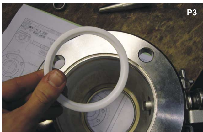
Remove the bottom ball seal from the valve body.
