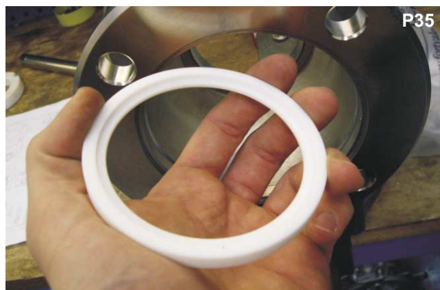
Ensure the back seal is in the correct orientation. Inspect the valve body for any dirt and foreign objects.
