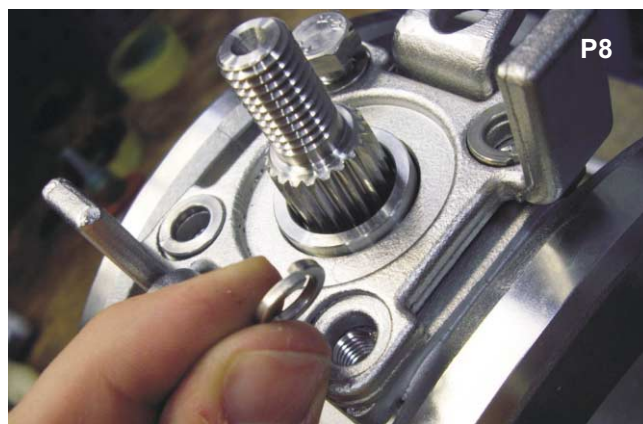
Remove the four M8 spring washers.
