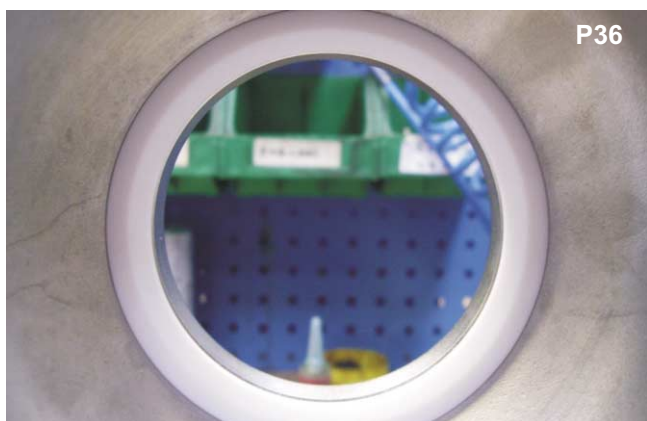
Ensure the back seal is fully located in the back groove.
