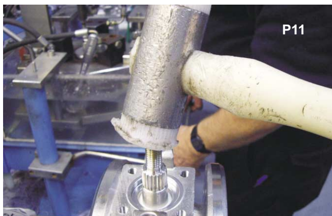
Gently tap the spindle to free from bore.
