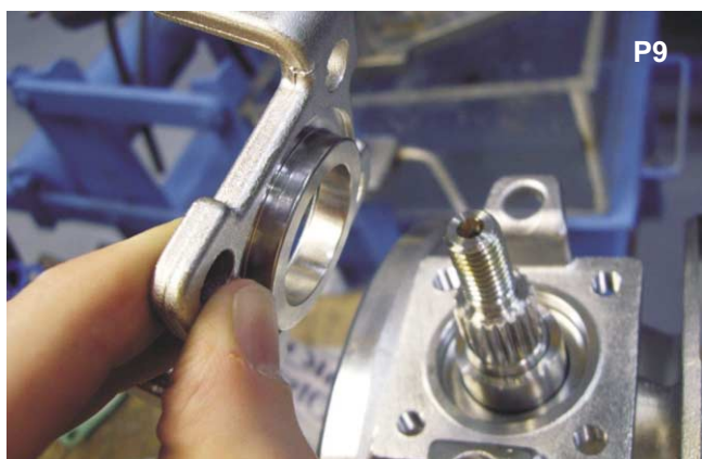
Remove the stuffing clamp.
