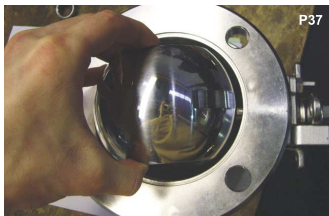
Roll the ball into the valve body.
