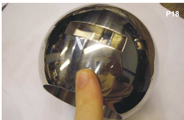
Check the ball for excessive wear, scratching or damage around the sealing areas at both ends of the ball.
