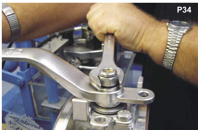
Holding the valve handle tighten up the M12 nut using a 19mm A/F wrench.
