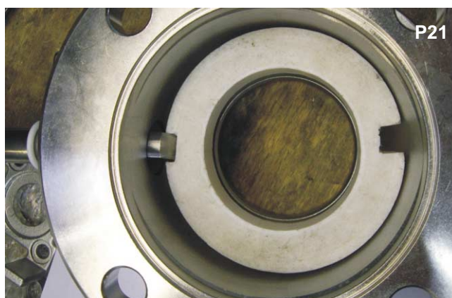
A tool like the one shown above (which is simply a 4.5" diameter piece of PTFE bar with a cut out for the spindle to locate on) must now be used to stop the spindle falling out.
