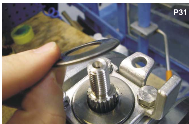
Replace the second Belleville washer dished side up as shown.
