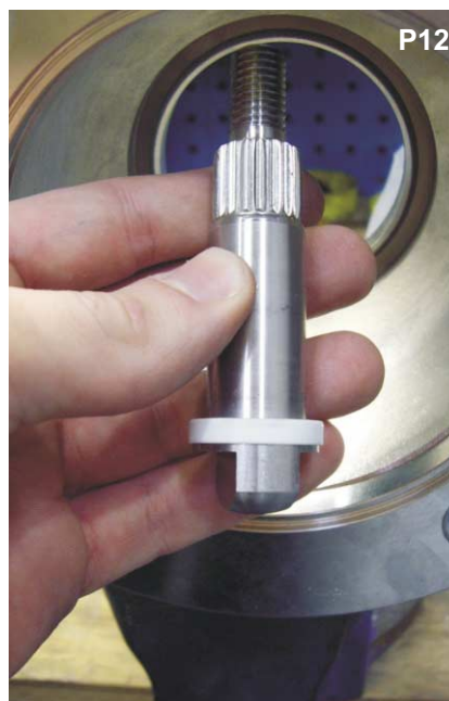
Once free from bore remove the spindle from the valve body.
