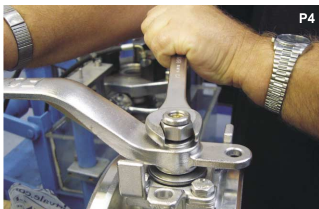
Holding the valve handle and using a 19mm remove the M12 lock nut.
