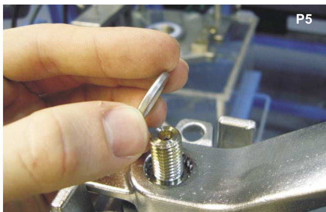
Remove the M12 washer.
