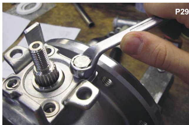
Using a 13mm wrench hand tighten the clamp plate bolts.
