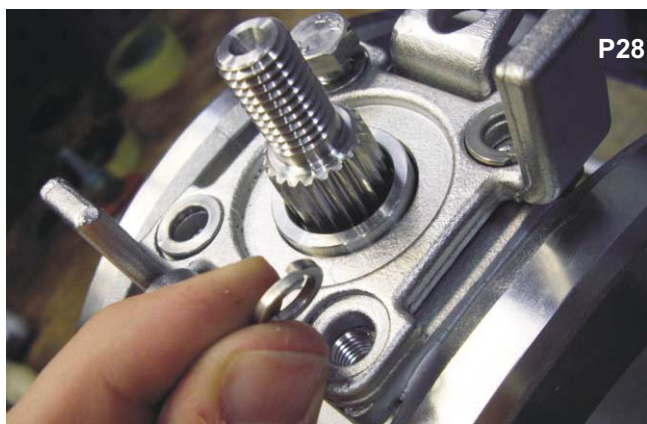
Replace the four M8 spring washers.
