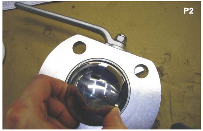
Using the ball valve handle, rotate the ball until the slot is inline with the axis of the valve. This will allow the ball to be carefully removed from the valve body.
