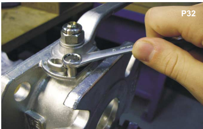
Replace the handle stop pin and tighten using a 10mm A/F wrench.
