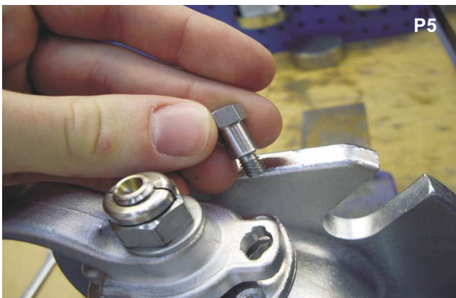
Completely remove the handle stop pin.
