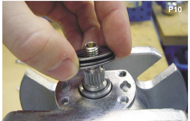
Noting the orientation of the Belleville washers remove from spindle.
