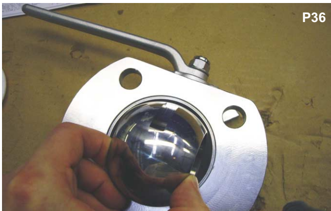
Roll the ball into the ball valve body ensuring that the flats on the ball spindle are inline with the ball valve axis.
