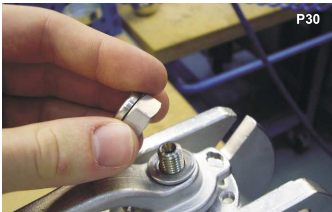
Replace the M10 self locking nut.
